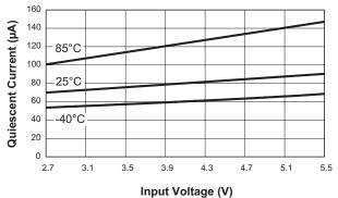
No Load Quiescent Current vs. Input Voltage (Step-Down Converter Enabled; Both LDOs Disabled)
