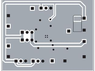
Figure 2: AAT2504 Evaluation Board Bottom Side Layout.
