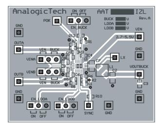
Figure 1: AAT2504 Evaluation Board Top Side Layout.
